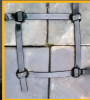
Correct way to use cable ties
